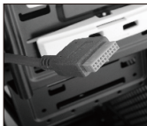
Internal USB 3.0 connector inside the case
